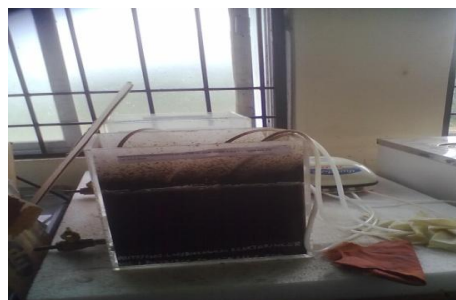
Figure 1 Fabrication of a Sequential Batch Reactor
